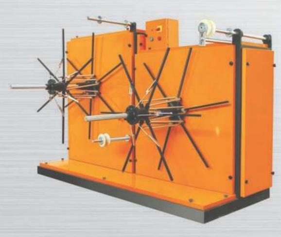
Volcano has developed adjustable gear motor operated two-spool winder, which winds pipe online. It winds pipe in coil from on spool as per out put available. Its extraction is made simply easy by umbrella design coil size can be of ID-Ø10", OD-Ø36", width-9" or as per customer requirements.
